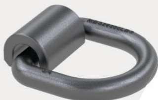
Part #LR-0750-R1-FC1 3/4" Weld On 26,500 lbs MBS
